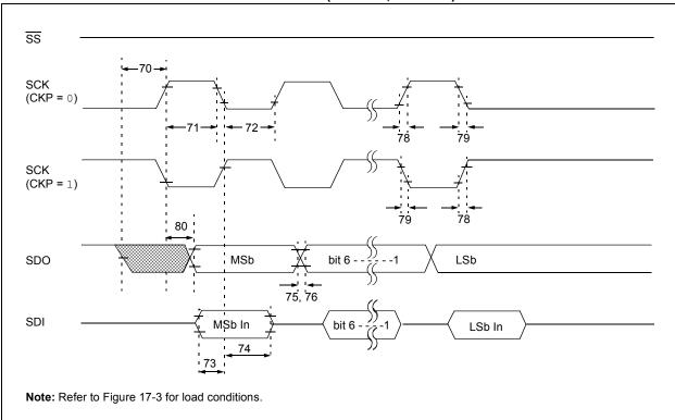
FIGURE 17-15: SPI MASTER MODE TIMING (CKE = 1, SMP = 1)
