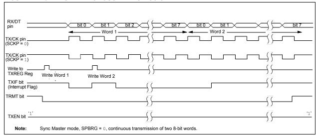
FIGURE 12-11: SYNCHRONOUS TRANSMISSION (THROUGH TXEN)
