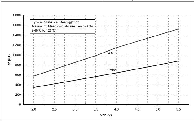
FIGURE 18-8: MAXIMUM IDD vs. VDD (EXTRC MODE)
