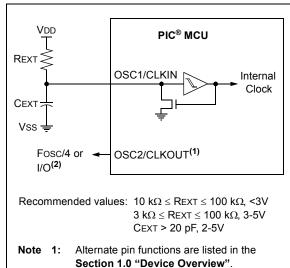
In RCIO mode, the RC circuit is connected to OSC1.
