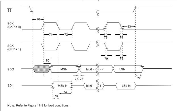
FIGURE 17-17: SPI SLAVE MODE TIMING (CKE = 1)
