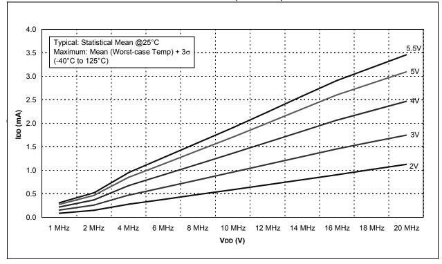
FIGURE 18-2: MAXIMUM IDD vs. Fosc OVER VDD (EC MODE)
