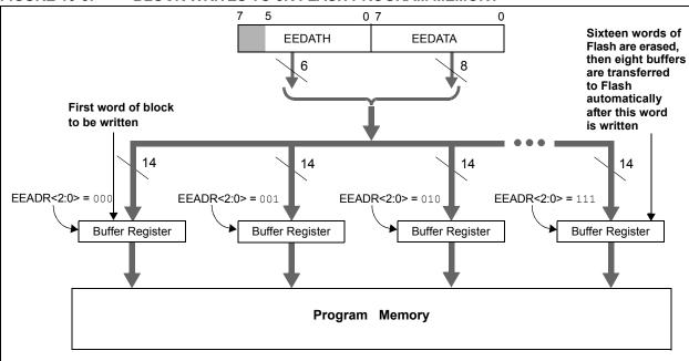
An example of the complete eight-word write sequence is shown in Example 10-4. The initial address is loaded into the EEADRH and EEADR register pair; the eight words of data are loaded using indirect addressing.
