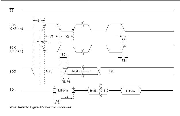
FIGURE 17-16: SPI SLAVE MODE TIMING (CKE = 0)
