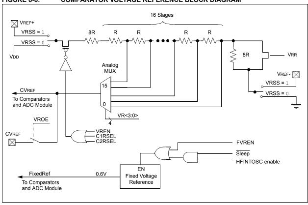
FIGURE 8-9: COMPARATOR AND ADC VOLTAGE REFERENCE BLOCK DIAGRAM
