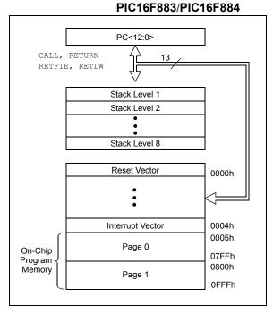
FIGURE 2-3: PROGRAM MEMORY MAP AND STACK FOR THE PIC16F886/PIC16F887
