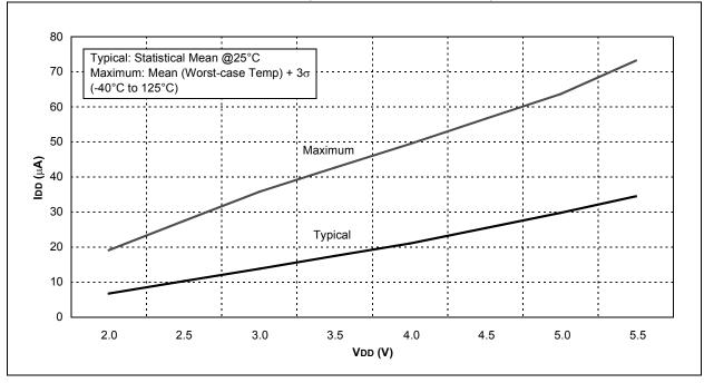
FIGURE 18-10: IDD vs. VDD (LP MODE)
