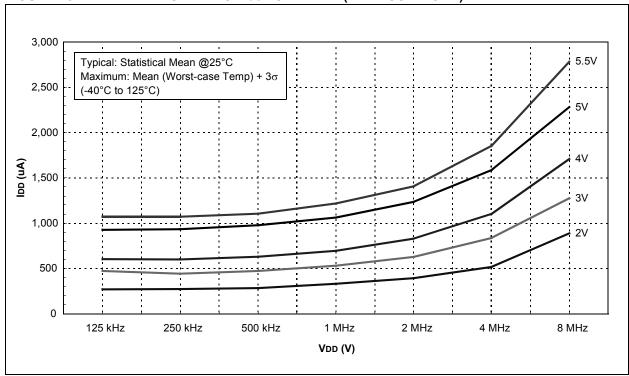
FIGURE 18-13: TYPICAL IPD vs. VDD (SLEEP MODE, ALL PERIPHERALS DISABLED)
