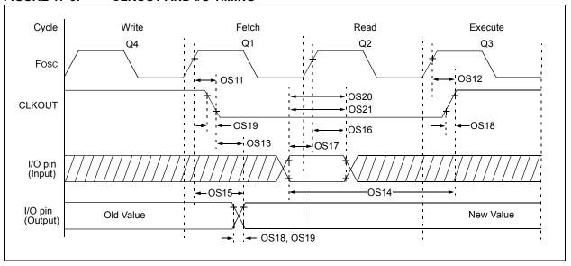
TABLE 17-3: CLKOUT AND I/O TIMING PARAMETERS
