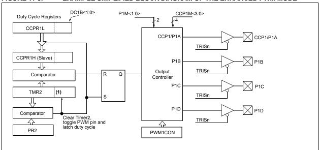
The 8-bit timer TMR2 register is concatenated with the 2-bit internal Q clock, or 2 bits of the prescaler to create the 10-bit
