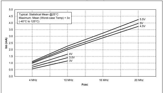
FIGURE 18-4: MAXIMUM IDD vs. Fosc OVER VDD (HS MODE)
