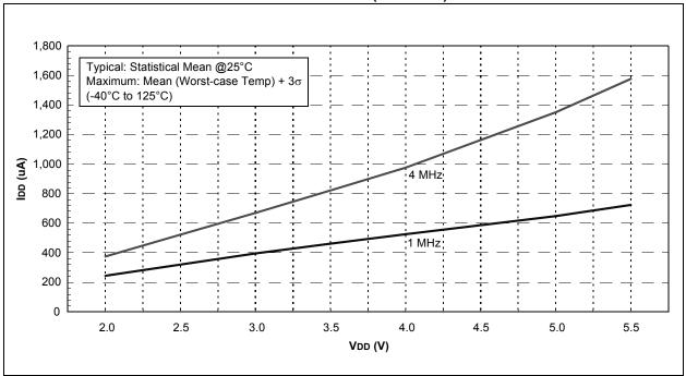
FIGURE 18-7: TYPICAL IDD vs. VDD OVER FOSC (EXTRC MODE)
