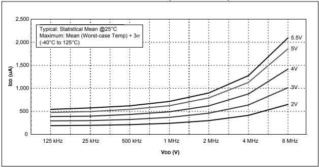
FIGURE 18-12: MAXIMUM IDD vs. FOSC OVER VDD (HFINTOSC MODE)
