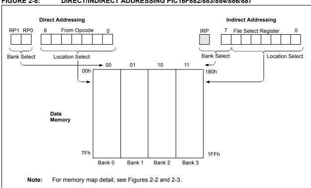
FIGURE 2-8: **DIRECT/INDIRECT ADDRESSING PIC16F882/883/884/886/887**
