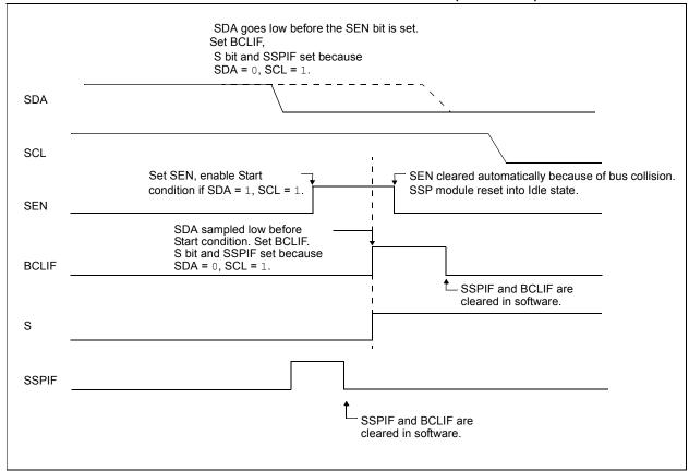
FIGURE 13-22: BUS COLLISION DURING START CONDITION (SCL = 0)
