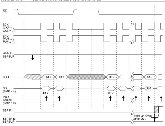
FIGURE 13-4: SPI MODE WAVEFORM (SLAVE MODE WITH CKE = 0)
