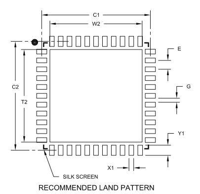
**MILLIMETERS** Units **Dimension Limits** MIN NOM MAX Contact Pitch 0.65 BSC Ε Optional Center Pad Width W2 6.80 Optional Center Pad Length T2 6.80 C1 8.00 Contact Pad Spacing C2 Contact Pad Spacing 8.00 0.35 Contact Pad Width (X44) X1 Contact Pad Length (X44) Y1 0.80 Distance Between Pads G 0.25
